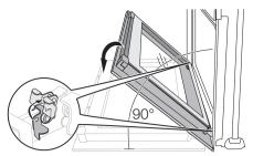
4. Fold the clamp levers on both door hinges (A) down into their original position.
